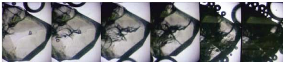
Fig. 6. Cracking and darkening followed by evolution of bubbles from a single crystal of DBSA . The entire sequence (from left to right) occurs in less than 20 s.
