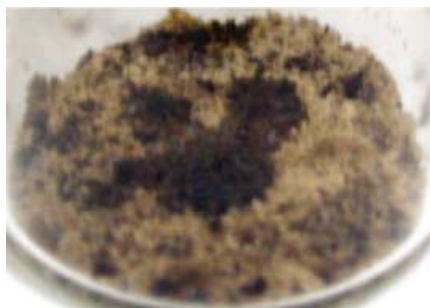
Fig. 10. Photograph of a sample of DBSA_{2/3}W containing both brown crystals and the beige material described in the text
